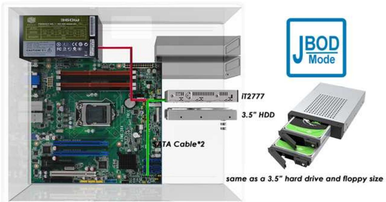
The iT2777 supports 6Gb SATA host interface and SATA 15 pin power supply. It allows 2x2.5" SATA drives to be fitted into 1x3.5" drive space, its size, SATA connector locations and screw holes are the same as 3.5" HDD. It provides JBOD feature and keeps OS and data separately in 2 HDDs/SSDs, so that users could upgrade it with RAID feature from installing a RAID adapter thru SATA cable.
